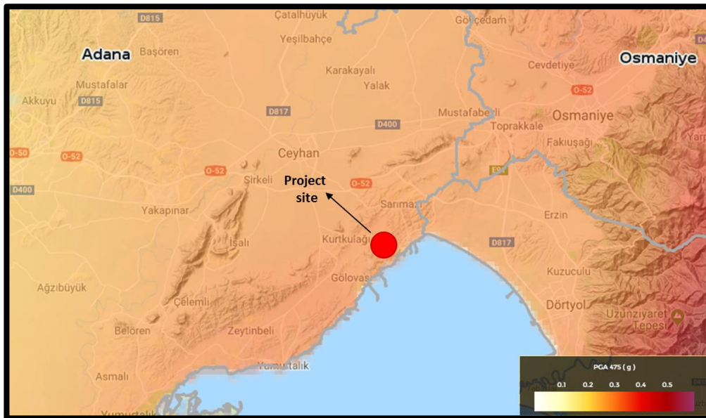
Figure 6-17. Earthquake Hazard Map for Project site and its close vicinity (Ministry of Interior Disaster and Emergency Management Presidency, 2019)
